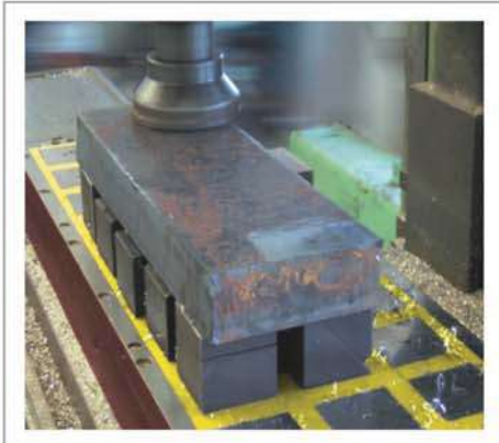
Side drilling and surface milling
