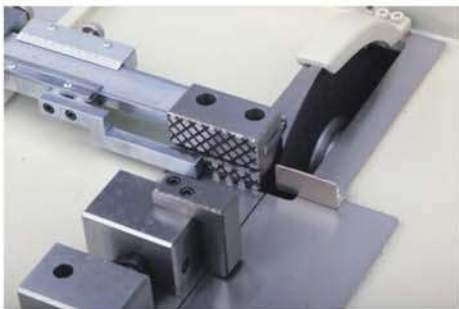
V shape clamping for round workpiece
